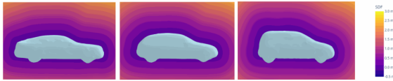
Fig. 42: The colored plane shows the respective points described through Signed Distance Function
