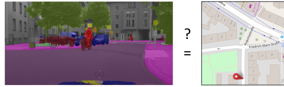
Fig. 37: Idea of street-map based validation, as proposed in [25]. The left image shows a segmentation of a traffic scene in the Cityscapes dataset [81] and the right image shows the corresponding map from OpenStreetMap [24]. In our approach, we employ such street maps to check the knowledge conformity of AI models.
